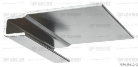
Steel 4/112 mm L-shape CF floor profile, S500, Magnelis-coating L=13140 mm 954.S412
