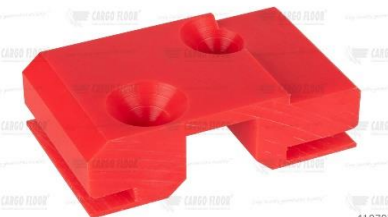
Solid red Anti Lifting guidance block for mounting over tube 25/25 mm for Cargo Floor steel L-shape floor profile (98x60x32 mm with 2 holes ø7 mm)
