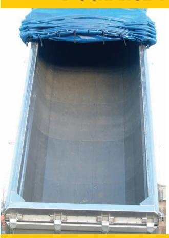
Harsh are a proud supplier and installer of the market leading Quicksilver Bodyliner. Quicksilver Bodyliner is designed for both rigids and trailers covering your tipper body floor and lower sides in one easy fit piece. It offers the highest ever resistance to internal abrasion, whatever
