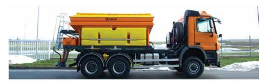
System for mounting the spreader in a tipper box using RO-RO (Roll-On, Roll-Off) legs and rollers on the device itself is the most common and simplest mounting method. The spreader is easily attached to the tipper box by using tension chains or belts.
