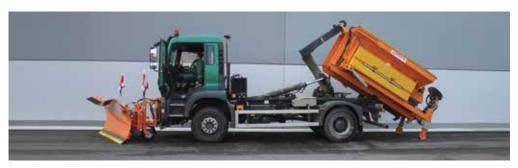
A specially adjusted spreader frame enables simple mounting on vehicles equipped with a system for raising devices using a hook.
