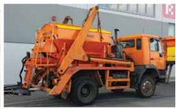
Simple mounting on vehicles equipped with a container lifting system is enabled by special attachment points on the sides of the spreader.
