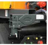
Fast and simple mounting using the existing sub-chassis of the vehicle tipper box and a special carrying frame on the spreader. The simplest mounting method that enables complete vehicle multifunctionality.
