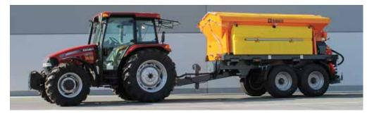
Spreaders are mounted on tractor or truck trailers, thus becoming independent from the towing vehicle.
