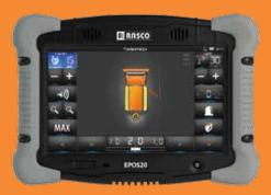
Enables automated road spreading based on the current location (GPS vehicle position), predefined routes of vehicle movement and predefined spreading parameters. By using the aforementioned parameters, the control unit automatically adjusts characteristics of the spreading pattern, such as width, asymmetry and quantity of spreading material.
