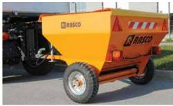
Mounting is performed by a rear hook or attaching the vehicle to the drawbar. The spreader is secured from side movements during reverse driving with chains attached to the vehicle box.
