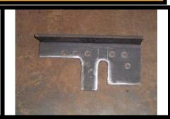
The position of the brackets will be shown on the layout assembly drawing. Care should be taken to ensure that no foul condition could take place with gearbox/chassis components.
