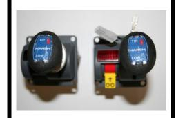
The Cab Controls Ports are cast into the sides of the cab control to ensure the cab control is correctly piped up.
