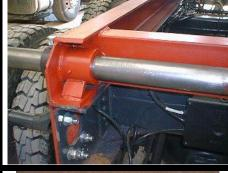
The ram and tank assembly is mounted to the chassis frame or chassis-reinforcing subframe by means of the Pedestal Bracket kit, fitted to the tank trunnion arms and mounted on the chassis/subframe members. The Pedestal Bracket kit consists of a bottom Pedestal bracket and a top Cradle bracket.
