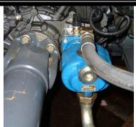
A suitable air supply should be located to enable the PTO engagement switch and cab control to be installed (the bodybuilder guideline booklet for your particular chassis will give a air location point).
