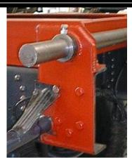
Ensure a suitable crossmember is fitted in front of the Hinge Bar. The Hinge Boss must also be fabricated with suitable gussets.
