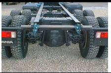
The hinge bar should be drilled and locked at the chassis bracket / boss points once the hinge bar is centralised.
