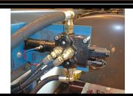
The system piping should follow the instructions in the fitting manual. The pipes should run as direct as possible with regular clamping and any bends required should be large natural curves to allow for hose compression. Always ensure **NO** hose is straight as this will pull the ends off the hoses when compressed. A body packer of 45mm will be detailed later, but care should be taken to ensure the power down pipes ( top ) DO NOT touch the lower cross tube.
