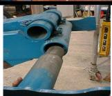
Place the assembled tipping gear on the chassis in the predetermined position. Centralise the Tipping Gear at both ends of the frame and make sure it is sat squarely on the Chassis.
