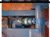
Pull out the top stage of the cylinder. Ensure the clamping ear is in the correct position with the short part towards the stabiliser knuckle.
