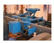
The low pressure feed from the tank to the pump should run along side the high pressure return from the pump to the valve.
