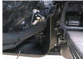
The tank return hose can now be fitted. Make sure if there is a curve in the hose it is not too loose / large as when under pressure it pulls upwards and touches the floor of the body.
