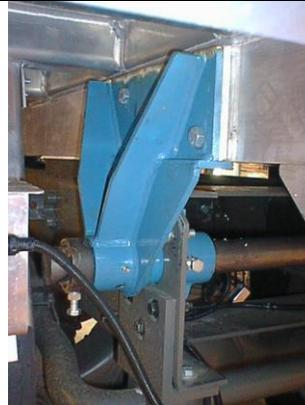
Once you have sat the body in position, before bolting to the body brackets ensure there will be no side movement from the hinge or body. Once bolted ensure the locking collars are fitted as shown with the bolt locked into the hinge bar. To achieve this you may wish to position the collar then through the tapped hole drill a pilot hole. Remove the collar and drill to suit the bolt size and depth remaining. Re-position the collar. Add locktite to the locking bolt and fix in place.
