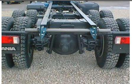
The hinge bar should be drilled and locked at the chassis bracket / boss points once the hinge bar is centralised.
