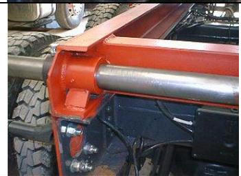
Liberaly apply grease to the clamping cup, circlip - again liberaly greased with the grease hole located in line with the grease nipple in the side of the cup.
