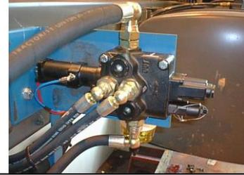
The system piping should follow the instructions in the fitting manual. The pipes should run as direct as possible with regular clamping and any bends required should be large natural curves to allow for hose compression. Always ensure **NO** hose is straight as this will pull the ends off the hoses when compressed. A body packer is required to ensure the minimum of 45mm pull out on the cylinder.
