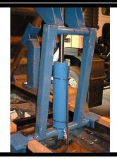
The tank should be filled with oil and then the system should be tested. Remember the rams have not been bled and there is no body attached at this point. Fully raise the tipper frame and then lower it back down. Do this 3 – 4 times to make sure the air is pushed fully out of the system. Re-fill the tank as required.
