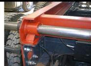
Place the tipping gear on the chassis in the pre-determined position. Centralise the Tipping Gear at both ends of the frame and make sure it is sat squarely on the Chassis.
