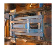
For mounting versatility the HARSH tipping gear can be mounted with the stabiliser standard or reverse.
