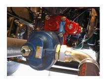
A suitable air supply should be located to enable the PTO engagement switch and cab control to be installed (the bodybuilder guideline booklet for your particular chassis will give a air location point).
